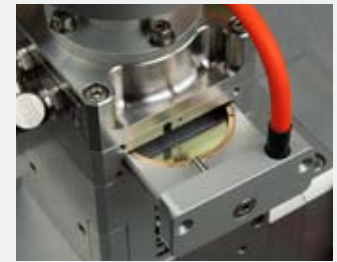
Cover Slide for additional protection of collimation
