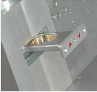
Exchangable cover slide for additional protection of the collimation module
