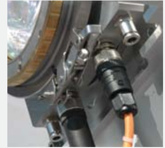
Electrical connection to integrated cover slide monitoring system
